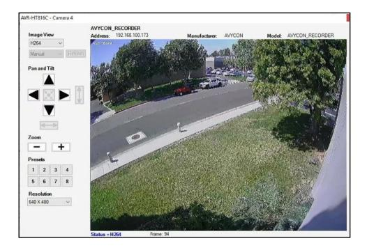
16. AVYCON recorder driver is communicating via API protocol, so before connecting to our recorder, please enter device GUI, and enable API server first, which is under network settings, below "port" menu. The authentication method is BASIC.
